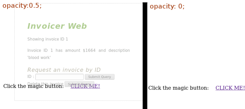
Figure 3.11 A clickjacking attack uses invisible IFrames, shown at 50% opacity on the left, to trick a user into clicking links to a target site.
