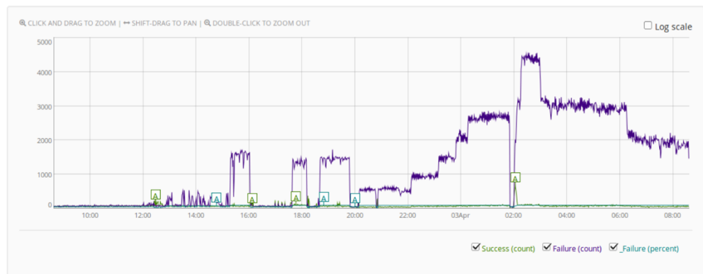
Figure 7.10 Monitoring graph to detect fraudulent logins on a sensitive service. Each letter A represents an anomalous increase of successful logins, which coincides with a large increase in failed login attempts.
