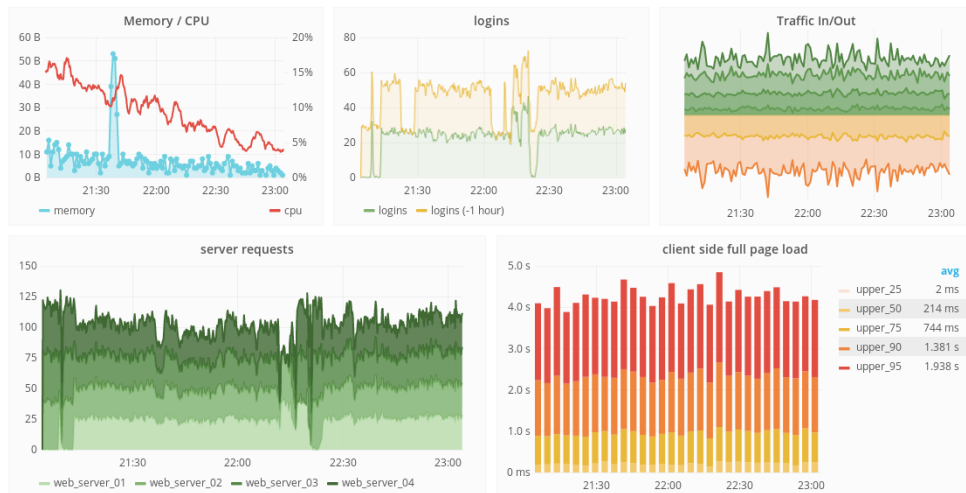
Figure 7.11 Grafana supports various types of graphs that are useful for rapidly conveying information across audiences. The ease of use of tools like Grafana make them good fits for the access layer of a logging pipeline.
